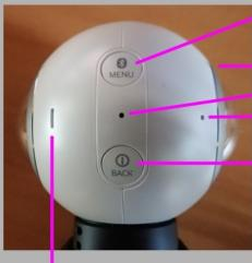
The menu button is used to navigate between the different settings. Can also be used for pairing Camera status Led
