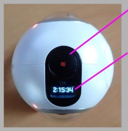
The top button is used to record a video or take a photo. It is also used to confirm the selected menu setting.
